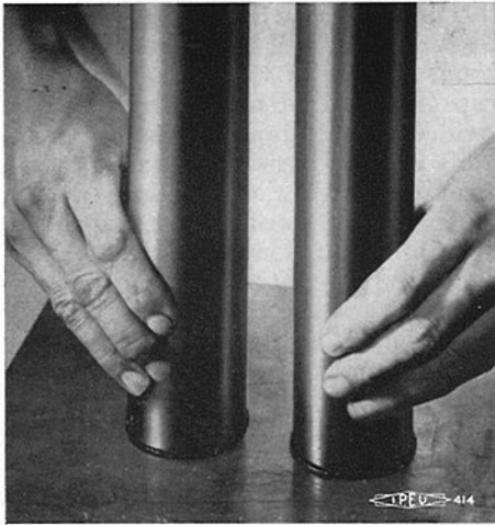
Place pieces to be welded on hot plate heated to 350-400° F. Hold until molten material inventory appears.
